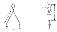
Material: Steel Finish: Electrogalvanized Static Load Safety Factor: 5:1
