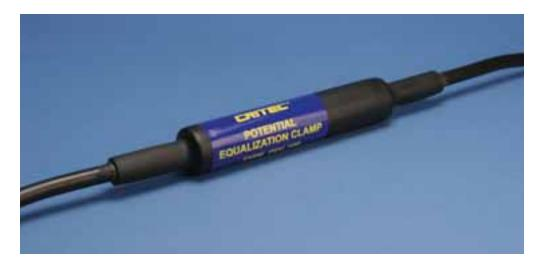
The PEC is an equipotential bonding device that is designed to minimize damage in applications where separated ground systems are required. The PEC100 model is ATEX approved making the device suitable for use in explosion hazard areas such as the protection of pipeline insulated joints. The PEC150 model is a higher surge rated product for more exposed locations subject to partial direct lightning strike.
