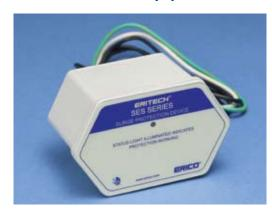
The SES40 Series of Surge Protection Devices provide economical protection against damaging transients and surge events. These products are UL and cUL® listed to 1449 Edition 3 as Type 1 devices. This allows them to be installed on the line or load side of the service panel in accordance with the NEC® 2011 without the requirement for additional circuit breakers or fuses. The DC models are listed under UL 1449 Edition 3 for Photovoltaic Systems.
