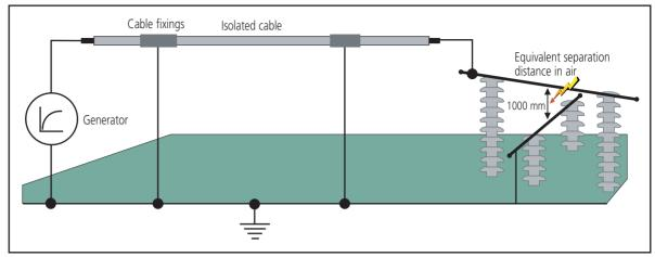
The isolated lightning protection detailed in IEC 62305 for the
