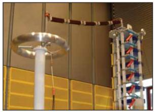
ERITECH Isolated Downconductor being tested
