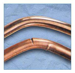
When an ERITECH® brand of copper-bonded ground rod (top) and a copper-clad rod are subjected to the same pressure load, the inferior copper-clad rod (bottom) develops cracks and creases to the outer sheath. Damage to the rod negatively affects its serviceable life and puts the integrity of the entire electrode at risk.
